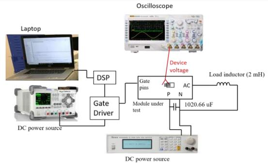
Fig. 21 Double pulse test setup.
