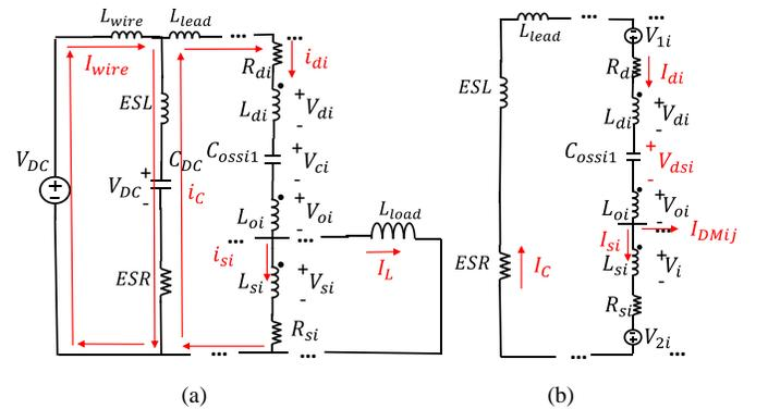
Fig.6 Equivalent circuits during the ringing stage: (a) time domain and (b) frequency domain.
