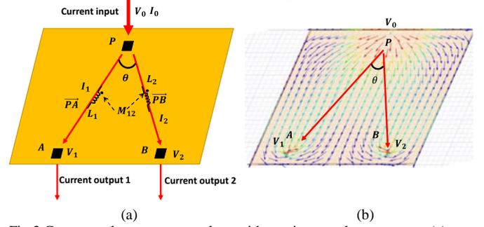
Fig.3 Current paths on a copper plane with one input and two outputs: (a) current paths, and (b) simulated current vectors.
