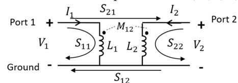
Fig. 16 Extraction of the inductance of two inductors with S-parameters.
