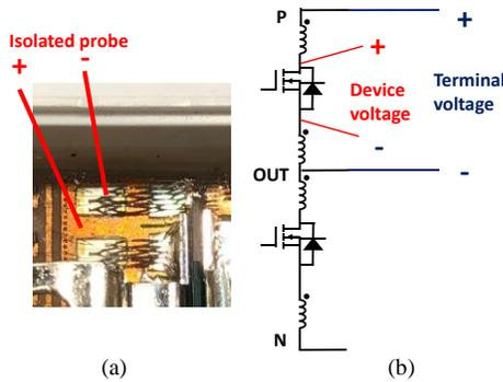
Fig.22 a) drain-to-source voltage measurement, b) circuit.
