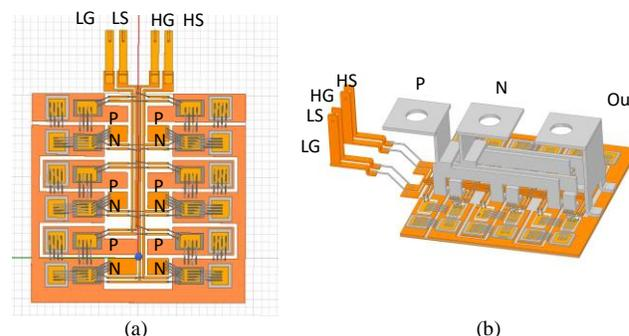
Fig.12 (a) proposed layout design with terminals hidden and (b) proposed module design with terminals.
