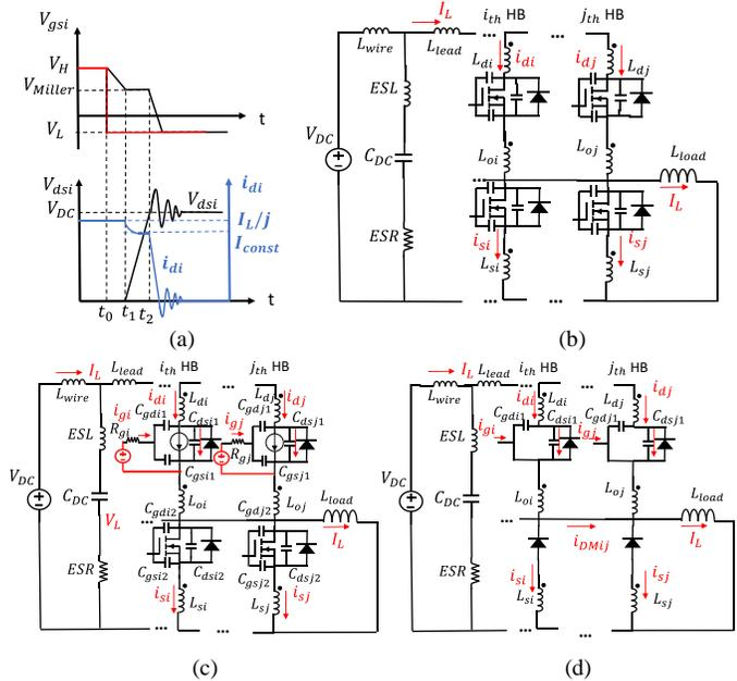
Fig.5 (a) The turn-off transient waveforms of the top switch and the equivalent circuits during: (b) stage 1, (c) stage 2 and 3 (d) stage 4.
