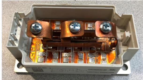
Fig.15 The prototype of the proposed HB SiC multichip power module.
