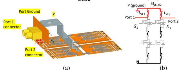
Fig. 17 Using two-port S-parameters to extract inductance with common ground connection: (a) ports and ground connections and (b) equivalent circuit.
