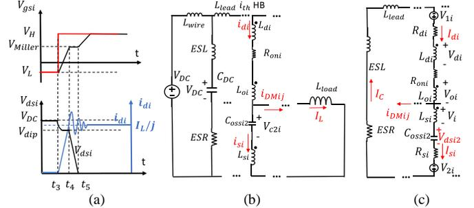
Fig.7 The turn-on transient of the top switch: (a) time-domain waveforms, (b) time-domain equivalent circuit and (c) frequency-domain equivalent circuit
