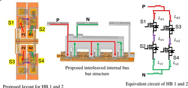
Fig. 11 The proposed module has small self and mutual inductances between two parallel HBs.
