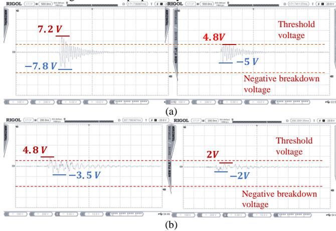
Fig. 24 Comparison of the measured gate voltage waveforms of the bottom switch when the top switch (a) turns on and (b) turns off.
