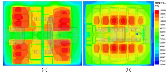
Fig. 26. Simulated temperatures of (a) original layout and (b) proposed layout.
