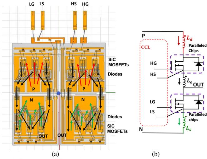
Fig.1 Commercial SiC multichip power module layout: (a) top view with the case and terminals hidden, (b) schematic with parasitic inductance.
