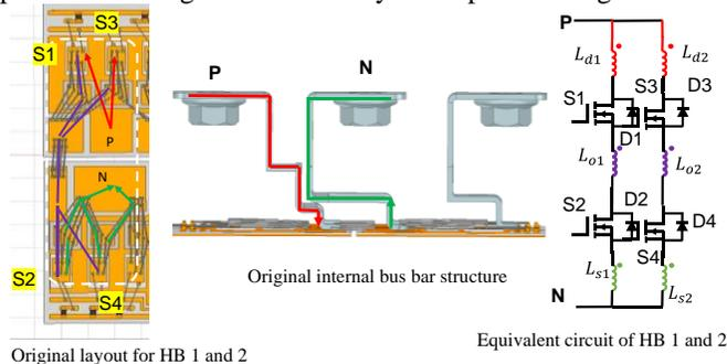
Fig. 10 The original module has large self and mutual inductances between two parallel HBs.
