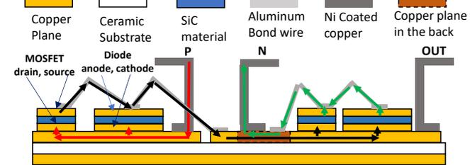
Fig. 2 Illustration of the three conduction path segments of the current commutation loop inside the power module with side view.
