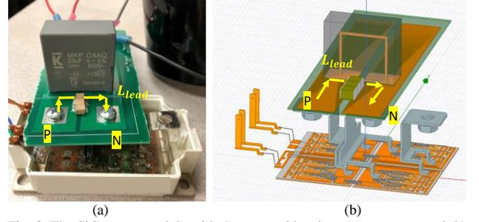
Fig. 8. The SiC power module with the external bus bar: (a) prototype and (b) 3D simulation model.
