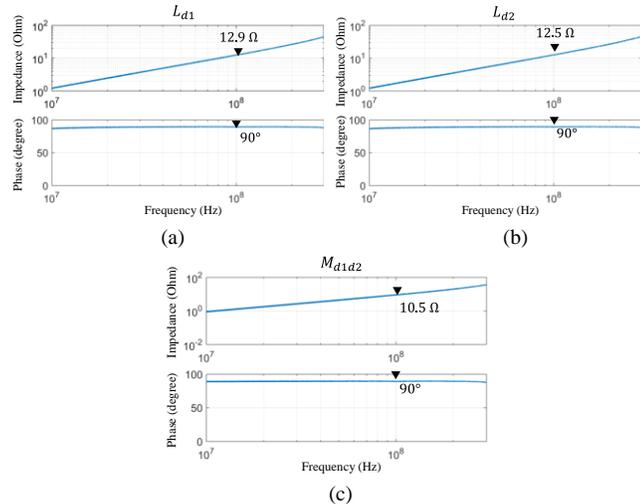
Fig. 19 Extracted impedance: (a)  $L_{d1}$ , (b)  $L_{d2}$  and (c)  $M_{d1d2}$ .
