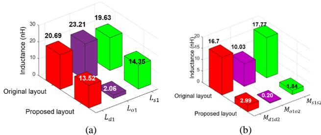
Fig. 20. Comparison of the measured self and mutual inductance of the two modules: (a) self-inductance and (b) mutual inductance.
