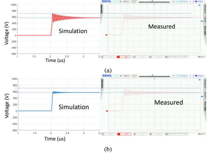
Fig. 9. Measured turn-off transient waveform compared with the simulated based on: (a) the proposed model (b) the model without mutual inductance.
