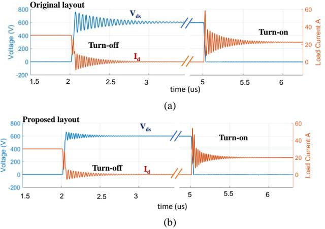
Fig. 25. Simulated switching waveforms during turn-on and turn-off transient for switching loss calculation: (a) Original layout (b) proposed layout.
