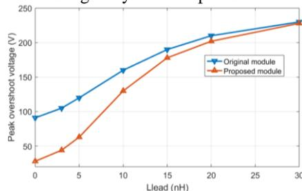
Fig.14 Simulated peak overshoot voltage comparison between the original module and the proposed module with different  $L_{lead}$ .
