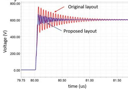
Fig.13 The comparison of the simulated drain-to-source voltage of the top switch during the turn-off transition between the original and proposed layouts.
