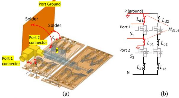
Fig. 18 Two-port S-parameters measurement with different ground connections: (a) ports and ground connections and (b) equivalent circuit.
