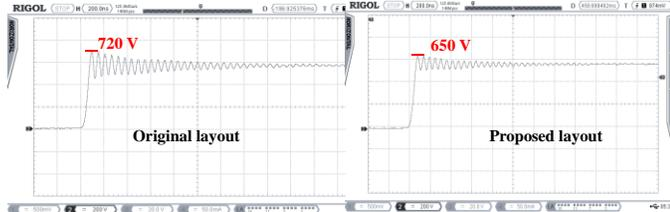
Fig.23. Comparison of the measured turn-off transient voltage waveforms between the original and the proposed layouts under a 600 V / 120 A test.
